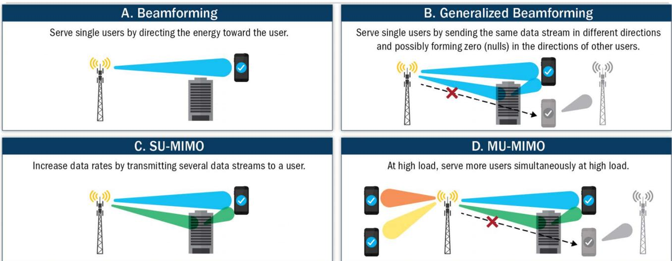
Figure 2. Advanced Antenna Systems – Beamforming and MIMO Examples<sup>16</sup>
